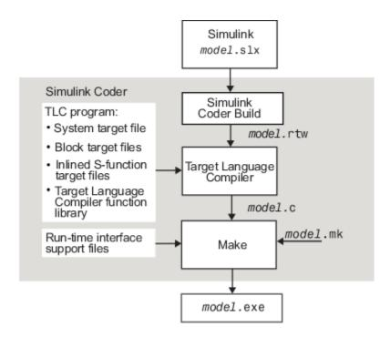
The Target Language Compiler (TLC) is designed to convert the model description file <code>model.rtw</code> (or similar files) into target-specific code or text.
